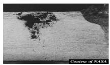
Figure 2. inter-grain Corrosion [10]
